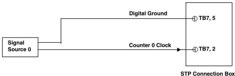
**Figure 20: Connecting Counter/Timer Signals to the STP Connection Box for a Continuous Edge-to-Edge Measurement Operation**
