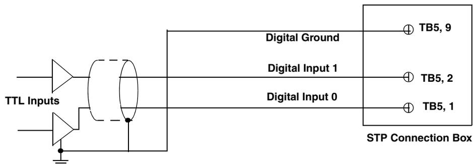
Figure 12: Connecting Digital Inputs to the STP Connection Box
