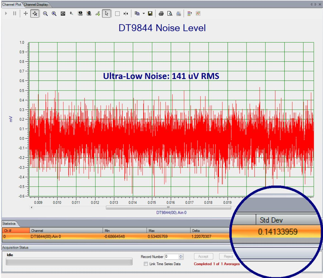
Figure 27: Typical System Noise of the DT9844
