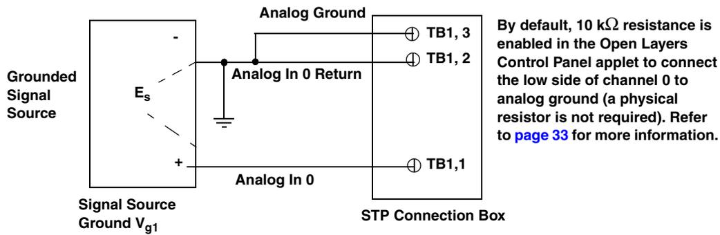
Figure 10: Connecting Differential Voltage Inputs from a Grounded Signal Source to an STP Connection Box
