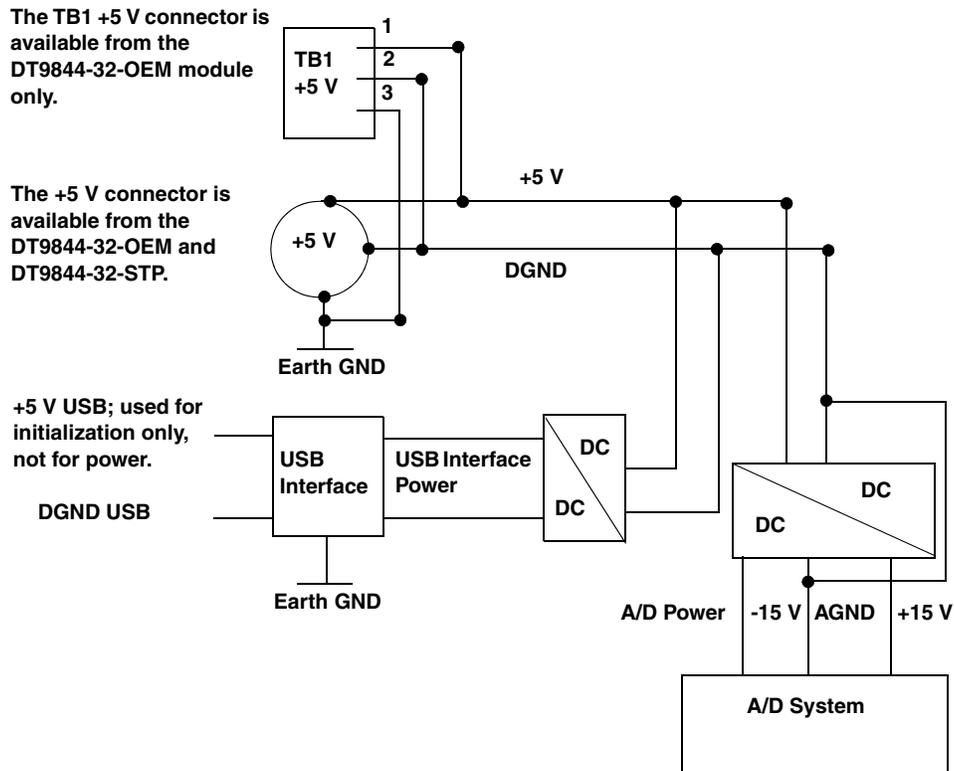
Figure 40: Ground, Power, and Isolation Connections
