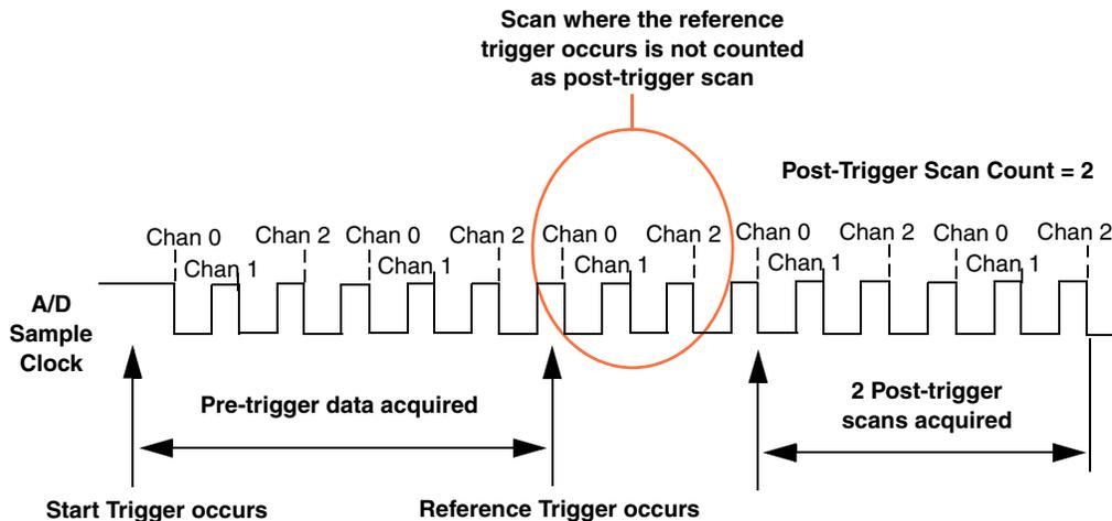
Figure 24: Continuous Scan Mode on a DT9844 Module Using a Start and Reference Trigger
