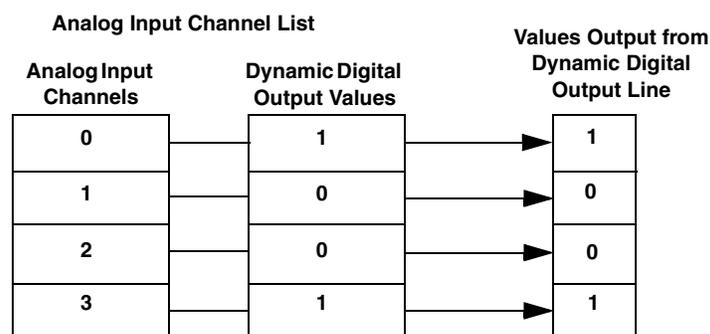
**Figure 23: Example Using Dynamic Digital Outputs**
