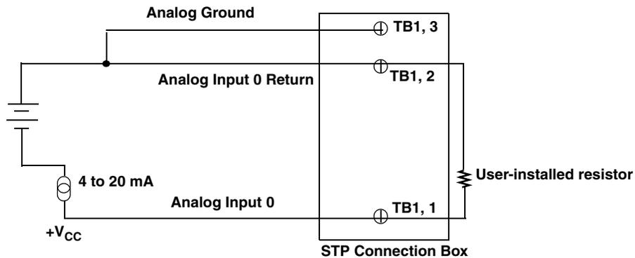
The user-installed resistor connects the high side of the channel to the low side of the corresponding channel, thereby acting as a shunt. For example, if you add a 250  $\Omega$  resistor and then connect a 4 to 20 mA current loop input to channel 0, the input range is converted to 1 to 5 V.
