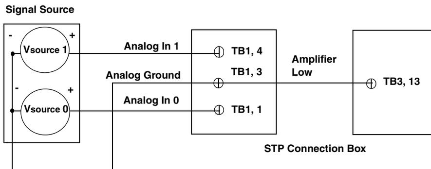
**Figure 7: Connecting Single-Ended Inputs to the STP Connection Box**
