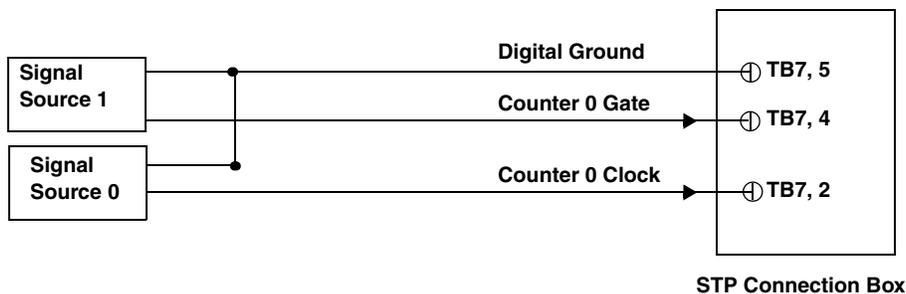
**Figure 19: Connecting Counter/Timer Signals to the STP Connection Box for an Edge-to-Edge Measurement Operation**
