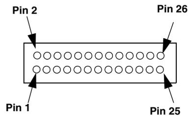
**Figure 31: Orientation of the Pins for Connectors J1 on the EP353 Panel**
