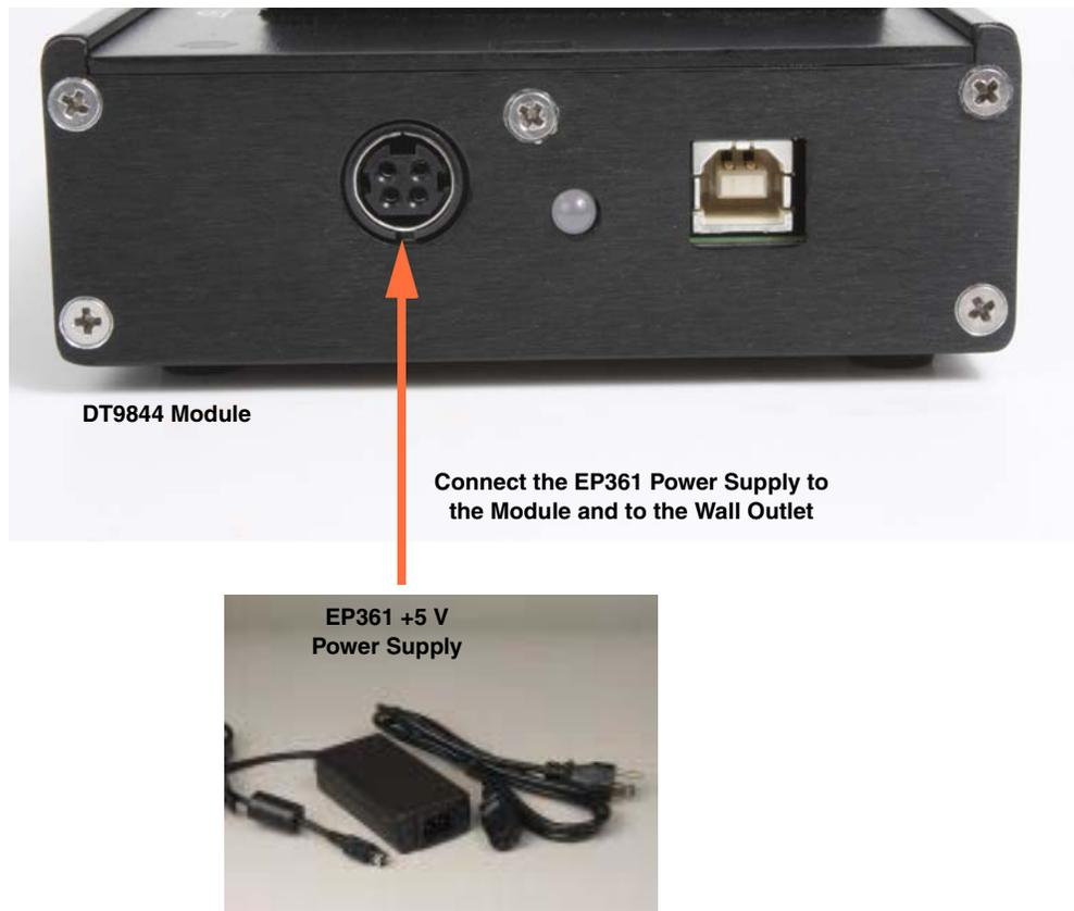
**Figure 3: Attaching a +5 V Power Supply to the DT9844 Module**
