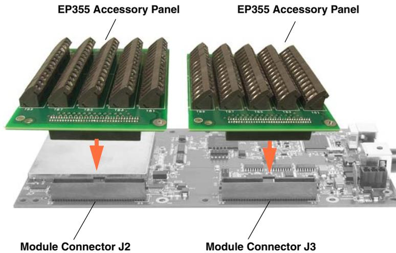
Figure 38: Connecting the EP355 Panel to the DT9844-32-OEM Module
