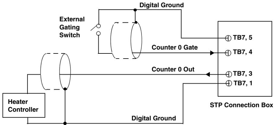
**Figure 21: Connecting Counter/Timer Signals to the STP Connection Box for a Pulse Output Operation Using an External Gate**
