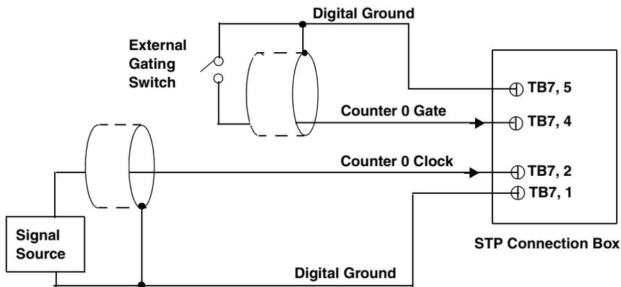
**Figure 14: Connecting Counter/Timer Signals to the STP Connection Box for an Event Counting Operation Using an External Gate**
