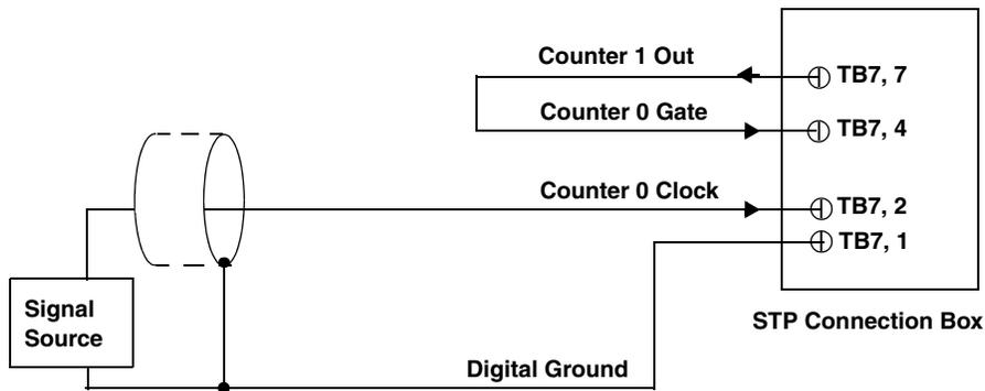
**Figure 17: Connecting Counter/Timer Signals to the STP Connection Box for a Frequency Measurement Operation Using an External Pulse**
