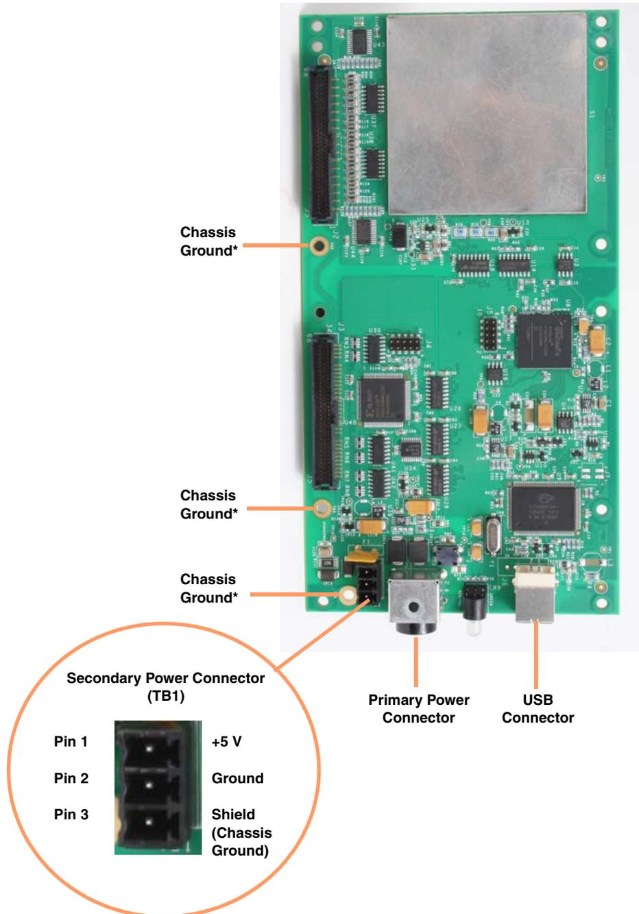
\*Note: All the holes that are unmarked are unconnected and can be used for mounting, if desired.
