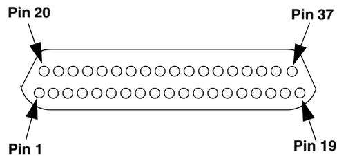
**Figure 35: Orientation of the Pins for Connectors J1 and J2 of the EP356 Panel**
