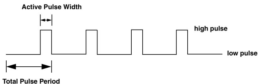
**Figure 26: Example of a Low-to-High Pulse Output Type**
