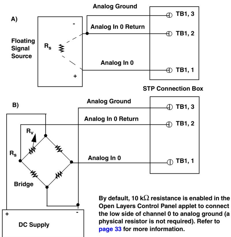
Figure 9: Connecting Differential Inputs to a Screw Terminal Panel
