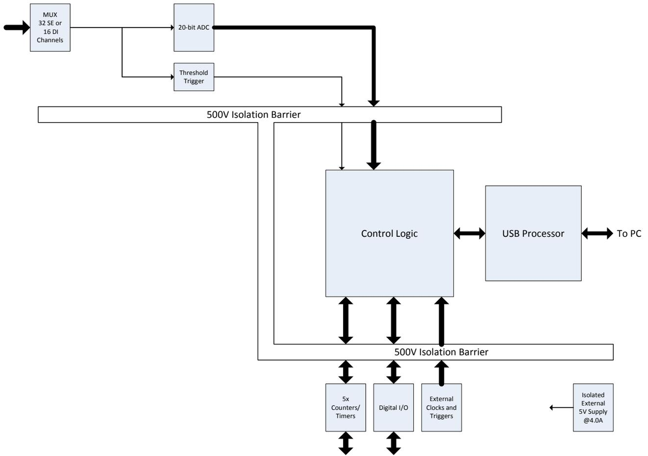
Figure 22: Block Diagram of the DT9844 Module
