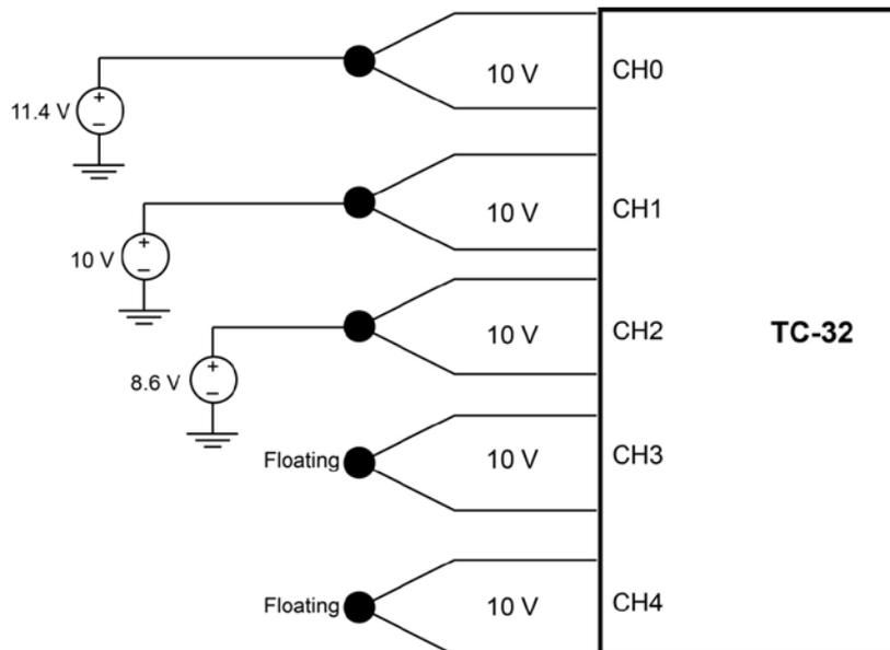
Figure 4. TC-32 common mode voltage connections example
