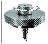
5 The probe shaft can be guided through the opening of the can and bottle attachment into the can or bottle.
