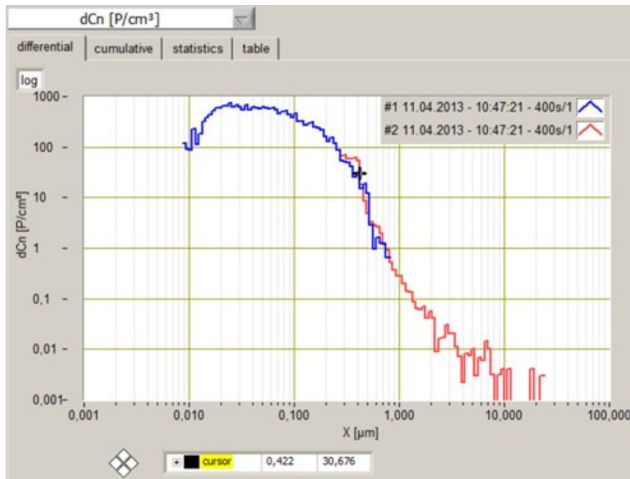
Figure 4: PDAnalyze evaluation software Measurement of indoor air concentration and display of number concentration Blue: Data from the U-SMPS, red: Data from the Fidas®
